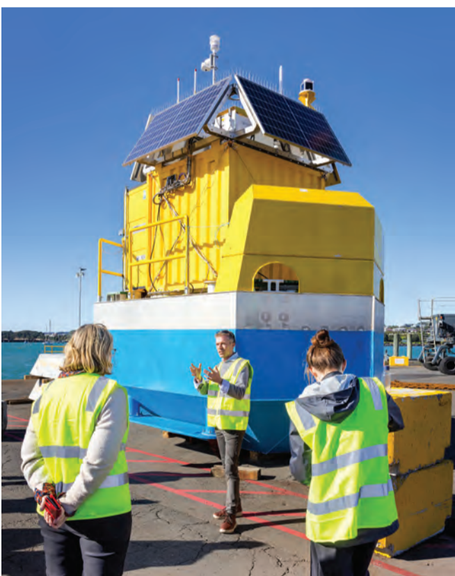
The Floating Light Detecting and Ranging (FLiDAR) device will measure wind, waves and currents and will be stationed in the South Taranaki Bight for one year.
