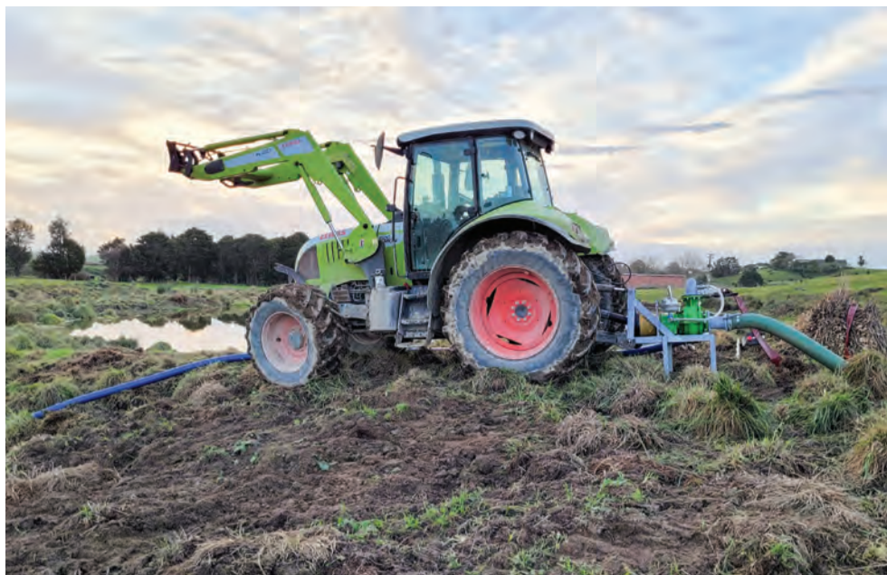
Tractor driven PTO pond stirrers can be taken to multiple storage areas
